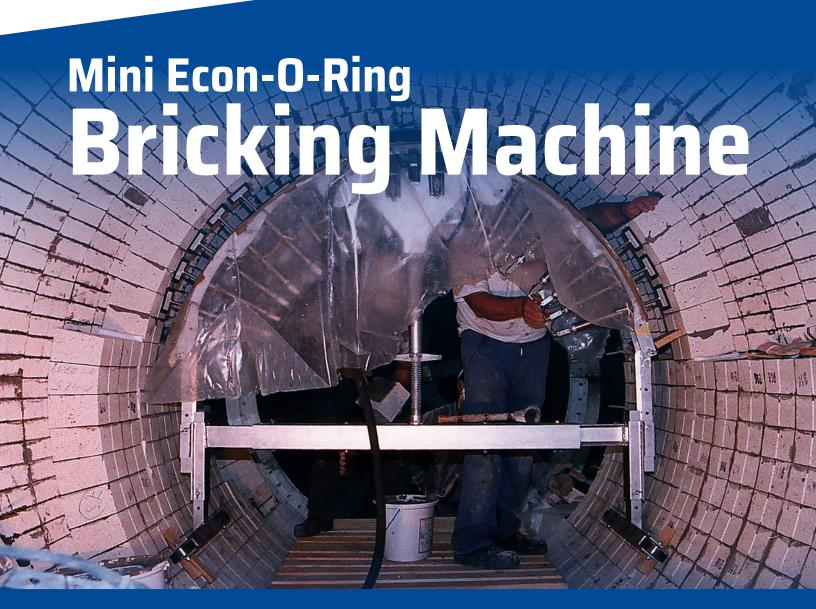
Smallest bricking machine for kilns with 1194mm - 2489mm (47"-98) Brick ID
